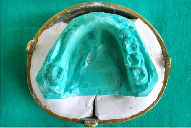
Fig 1: Fracture of investment material after elimination of wax
