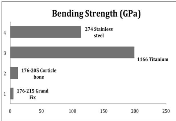
Figure 1- Bending strength of the material (according to manufacturer)
