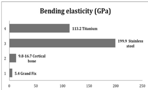
Figure 2- Bending elasticity of the material (according to the manufacturer)
