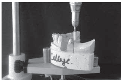
Fig 4: Preparing a 6 taper using surveyor and milling machine
