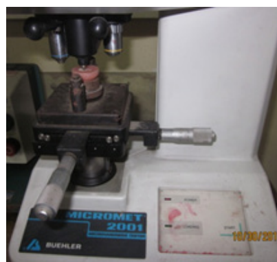
Figure 7: Indentation test in microhardness testing machine
